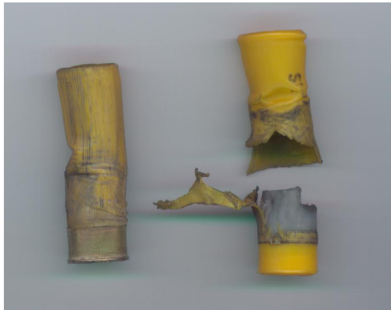
Fig 2. Typical debris from 20 bore cartridges recovered from down range showing a cartridge that had not fired and one that had fired.
